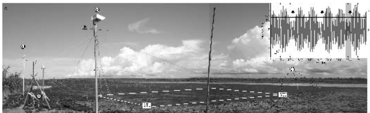
Figure 2: A/ Instrumentation in the study site. The white rectangle covers the surface extracted from photographs between station 1 (ST1) and station 2 (ST2). A: DGPS point, B: camera, C: scales along a transect, D: weather station. B/ presents the tide levels from 1/10/2008 to 4/09/2008. Black stars denote CDOE \geq 5 at a 2.67 m. elevation.
