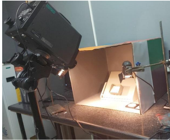
Figure 1. Geometry of spectral reflectance measurement using the spectrophotometer.
