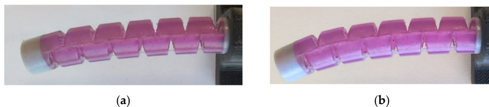
Figure 19. Fatigue test results: flexible element condition after (a) 400 and (b) 500 bending cycles.
