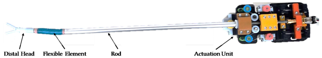
Figure 15. Prototype of the flexible laparoscopic instrument.
