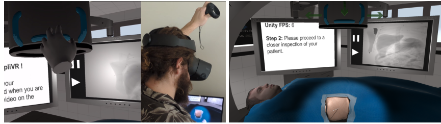
Figure 5: Inside the simulator : The user moving the C-arm (left). The OR environment with the fluoroscopic imagery on the right screen, and the patch of skin at the bottom. (right)
