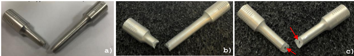
Figure 6. Optical Observation of the Fracture Surface of the Reference (a), and Samples Containing 500 µm (b) and 1 000 µm Pore (c)
