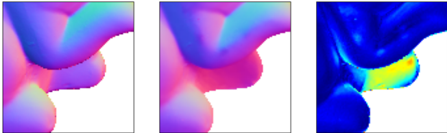
Fig. 3: Ground truth normals, estimated normals and angular error map. High errors are concentrated on the cast shadows areas.
