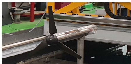
(a) 3-bladed turbine model fixed on its bottom mounting, out of water.
