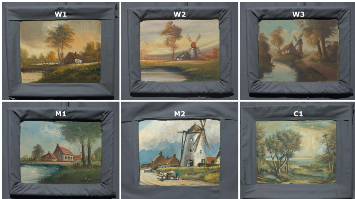
Fig. 3. Six test oil paintings on canvas evaluated during the experiment under the high-fidelity spectrum f_{95g_{100}} . Images are transformed to a daylight appearance by applying a von Kries chromatic adaptation transform from the 3000 K white point under illumination f_{95g_{100}} (as measured on a white patch of a Macbeth ColorChecker) to CIE D65. Regions outside the fixed visible area of 48 cm \times 39 cm were covered with mid-gray cloths to serve as background.
