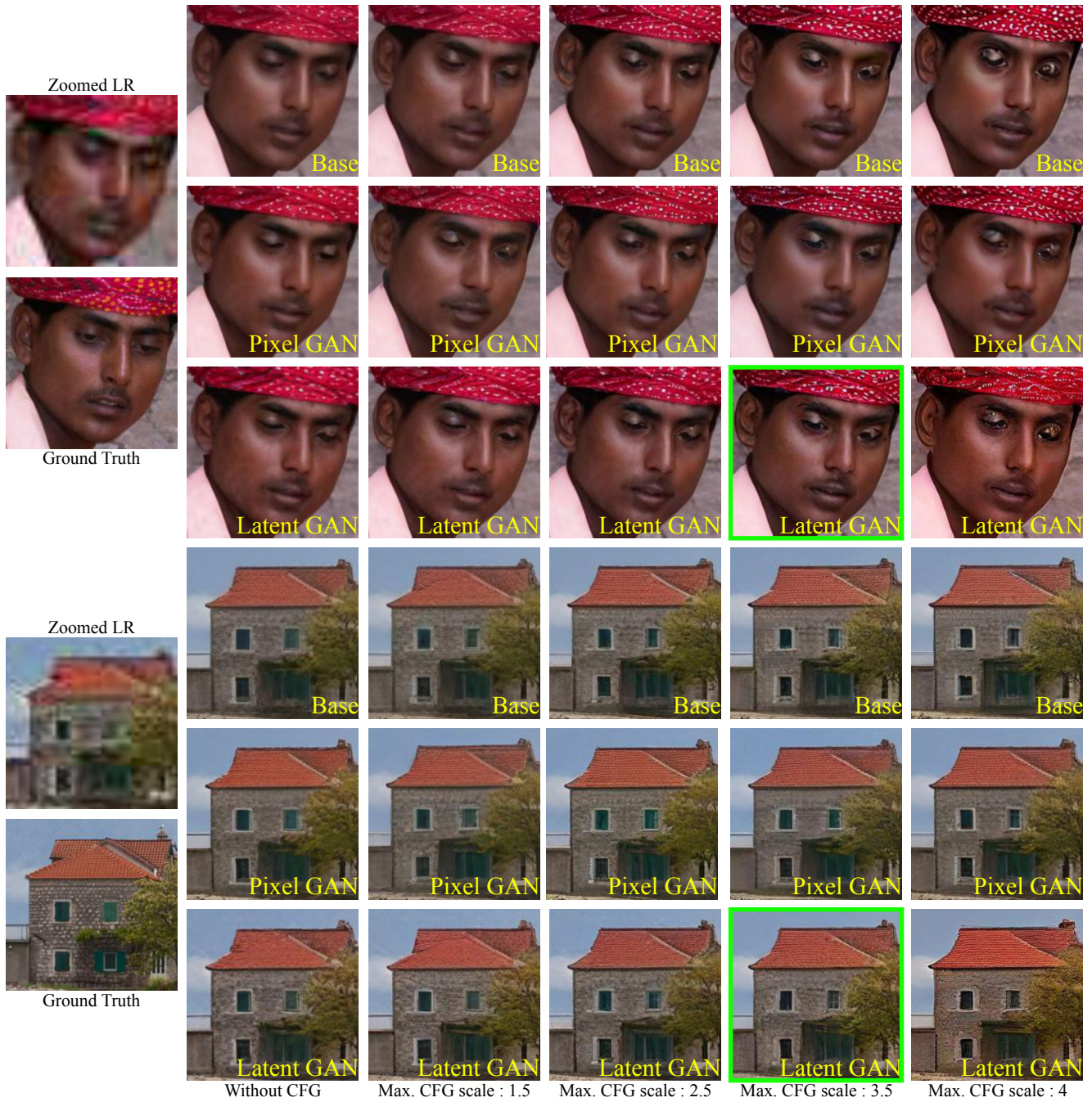
Figure 16: Qualitative comparison of adversarially finetuned Shortcut variants of FlowMapSR for \times 4 upscaling. The green setting ( w_{\max} = 3.5 & latent RPGAN) is the default configuration used in our main experiments. The LR images are taken from the Div2K-Val dataset. For each LR–HR pair, increasing the CFG scale alone (first row) already leads to noticeably sharper results, reflecting improved perceptual quality. When adversarial fine-tuning is additionally applied, texture fidelity and sharpness further improve. This effect is especially pronounced when fine-tuning is performed in latent space (third row), whereas pixel-space fine-tuning yields only marginal gains (second row). Overall, combining CFG with latent adversarial fine-tuning produces superior visual results compared to using solely CFG or adversarial fine-tuning on the standard FlowMapSR model.
