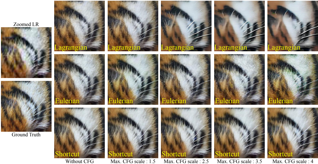
Figure 2: Qualitative comparison of positive-negative CFG enhancement applied to LSD-, ESD-, and SSD-based FlowMapSR for \times 4 upscaling. The HR reference image exhibits sharp edges and rich high-frequency details. The base FlowMapSR model (“Without CFG”) successfully recovers structural details but lacks perceptual sharpness. Applying positive–negative CFG improves visual realism in the Shortcut formulation (e.g., more natural hair textures), while it introduces noticeable degradations and artefacts in the Lagrangian and Eulerian formulations.
