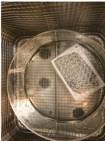
Ultra-sonication bath: microplate in a beaker contained ice cold water
