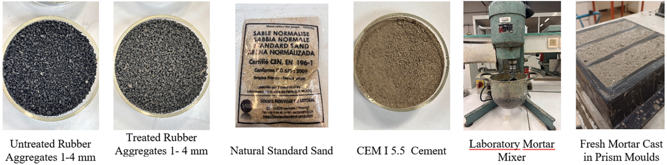
Fig. 3. Materials and equipment used for mortar production.
