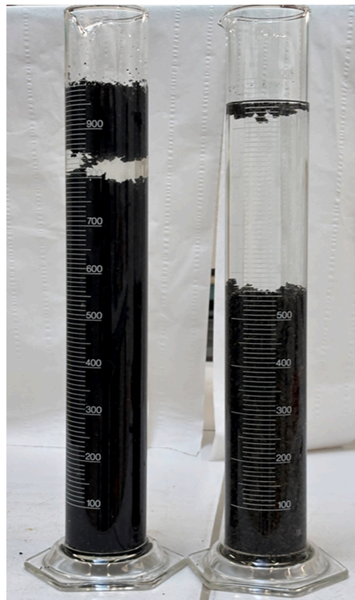
Fig. 2. Density and wettability of untreated and treated rubber aggregates.
