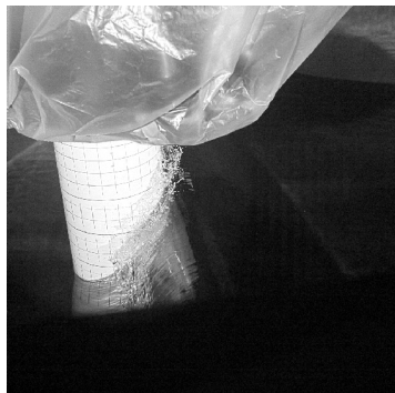
Figure 8: Images of wave 3 impacting the mockup for various values of \bar{\delta} . All the images are taken at the instant at which the impact load is maximum. The plot in the upper left corner corresponds to the numerical free-surface profile at the same instant. The solid vertical line indicates the position of the front face of the cylinder. The dashed vertical line indicates the position of the locally vertical front.
