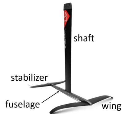
Figure 1. Olympic Class windfoil: IQFoil. Note the curved span of the main wing and the drooped tips.
