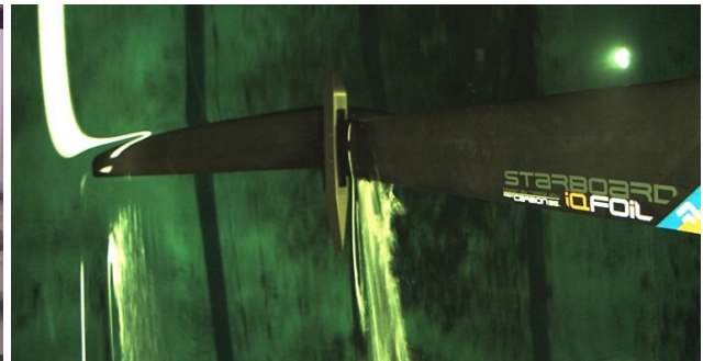
Figure 8. Ventilation on the wing piercing the free surface. (left) Full ventilation for heel angle \theta = 20^\circ , h/c = 0.75 , \alpha = 6^\circ , U = 7 \text{ m s}^{-1} ; (right) Partial ventilation for \theta = 30^\circ , h/c = 1.25 , \alpha = 4^\circ , U = 7 \text{ m s}^{-1} .
