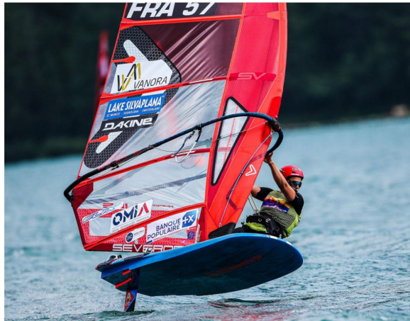
Figure 1. Olympic Class windfoil: IQFoil. Note the curved span of the main wing and the drooped tips.
