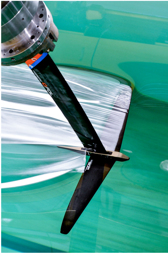
Figure 8. Ventilation on the wing piercing the free surface. (left) Full ventilation for heel angle \theta = 20^\circ , h/c = 0.75 , \alpha = 6^\circ , U = 7 \text{ m s}^{-1} ; (right) Partial ventilation for \theta = 30^\circ , h/c = 1.25 , \alpha = 4^\circ , U = 7 \text{ m s}^{-1} .
