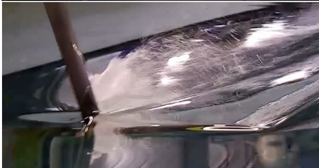
Figure 9. No ventilation case although the wing pierces the undeformed free surface at rest, for heel angle \theta = 20^\circ , h/c = 0.875 , \alpha = 4^\circ , U = 7 \text{ m s}^{-1} . Top left: front view at rest; top right: top view at speed; bottom left: front view at speed; bottom right: rear view at speed.
