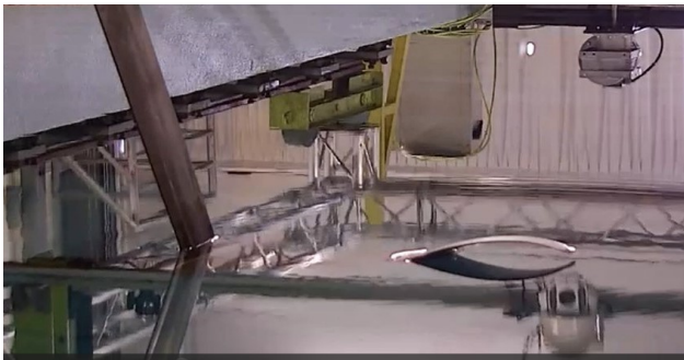
Figure 8. Ventilation on the wing piercing the free surface. (left) Full ventilation for heel angle \theta = 20^\circ , h/c = 0.75 , \alpha = 6^\circ , U = 7 \text{ m s}^{-1} ; (right) Partial ventilation for \theta = 30^\circ , h/c = 1.25 , \alpha = 4^\circ , U = 7 \text{ m s}^{-1} .
