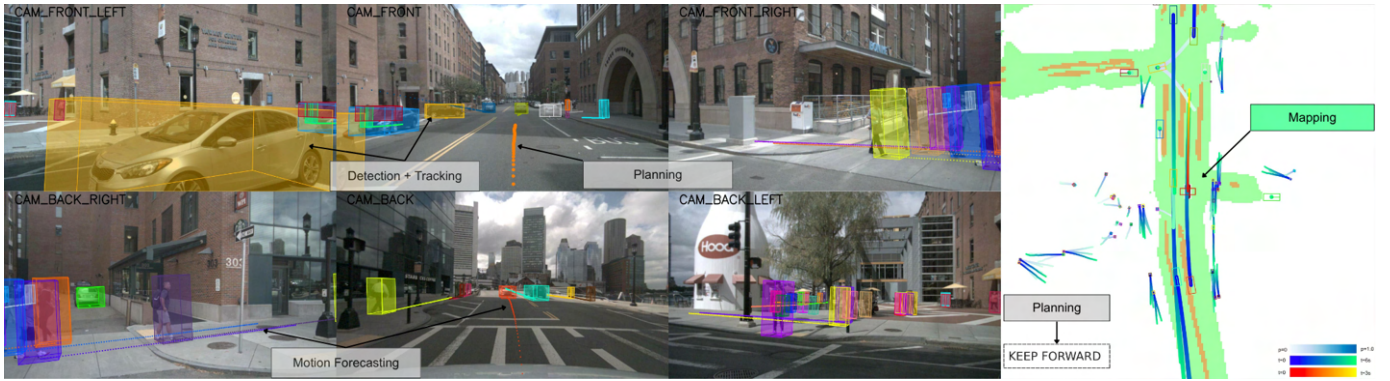
Fig. 2: Qualitative results of the OmniNAV system on a nuScenes example. The six synchronized multi-view camera inputs illustrate perception outputs including 3D object detection, tracking, and motion forecasting for surrounding agents, along with the planned trajectory of the ego vehicle. The right side shows the unified BEV representation combining detection, tracking, mapping, and trajectory planning, demonstrating consistent spatial reasoning across modalities.
