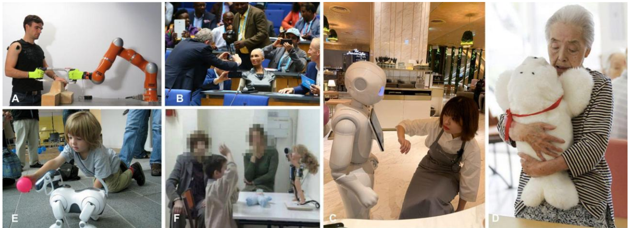
Figure 2: Examples of successful development of robots for human-robot interaction: (Top left) Collaborative robot (cobot) can support users in industrial tasks; (Bottom left) the Sony AIBO dog capable of learning users' preference through reinforcement learning driven by the user's pat on its head. (Middle top) Androids push the frontiers of how human appearance can be; (Middle bottom and far right) toy robots can be programmed to support rehabilitation programs, such as Robota (EPFL) for children with autism spectrum disorders, or the Paro seal robot used with the elderly suffering from dementia. (Middle right) Humanoid robots such as Pepper can serve as guides in museums or order and serve dishes in fast food.
