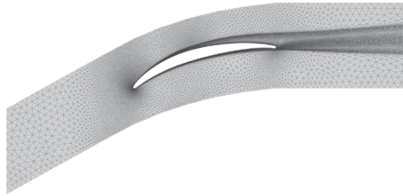
Fig. 7 LRN-OGV cascade: adapted mesh (based on the SA-BCM model) of complexity \mathcal{N}_c = 16\,000 and composed of \mathcal{N}_e = 38\,000 cells
