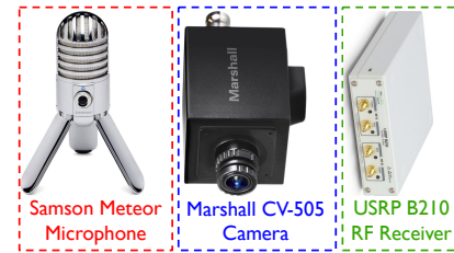
Figure 16: Sensing equipment used during the experiments.
