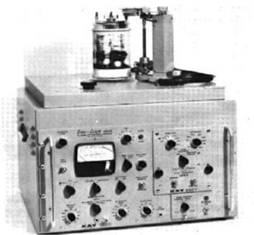
Figure 6. Kay Elemetrics Spectrograph « Sonagraph » (photo Kay Elemetrics)
