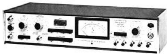
Figure 5. Melody detector with manually switched filters (Fundamental Frequency Meter, Frøkjær-Jensen Electronics).
