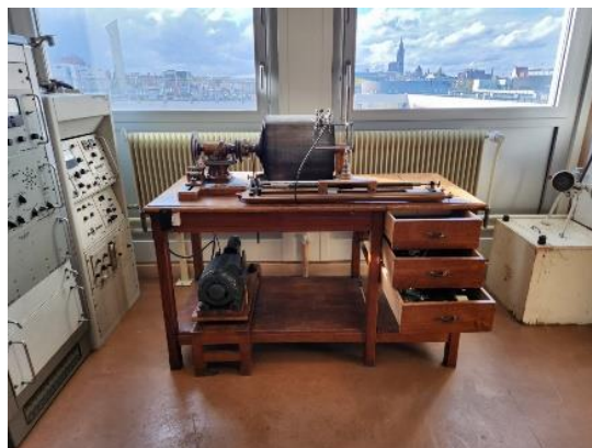
Figure 2. A photo showing the phonetic kymograph as supplied to The Phonetics Institute of Strasbourg, together with its accessories by G. Boulitte around 1947.
