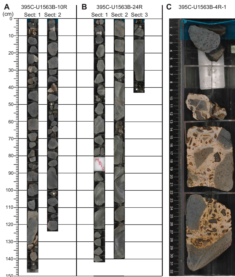
Figure F12. Common lithologies, Hole U1563B. A. Pillow lavas with occasional peperite fragments. B. Sheet flows. C. Peperite fragments exhibiting quenched glass rims, baked and partially crystallized sediment, fluidal margins, and other indications of lava-sediment interaction.
