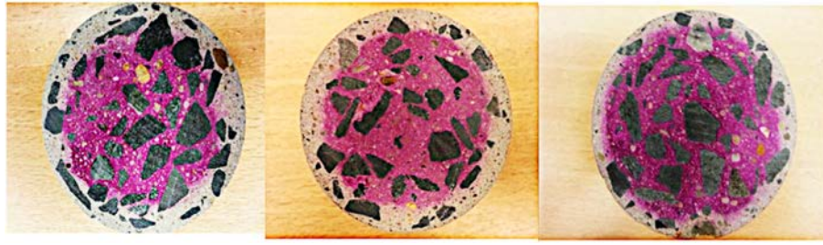
Fig. 19. Carbonated depths after 6 months of exposure, from left to right: t_0 = 16 h, t_0 = 24 h and t_0 = 48 h.
