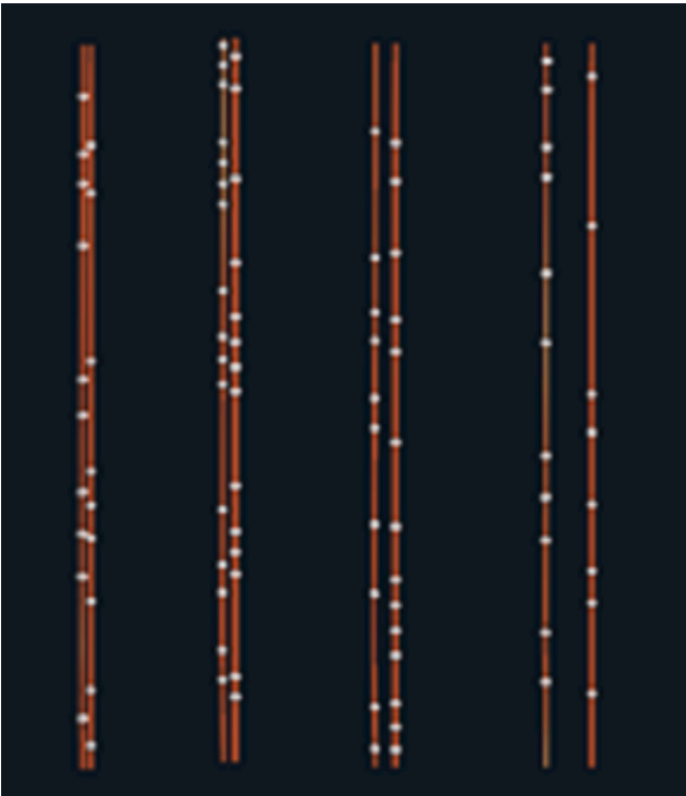
Fig. 1. Phantom of two linear vessels (red) for four different lateral separations: 100 \mu\text{m} , 200 \mu\text{m} , 400 \mu\text{m} , and 1000 \mu\text{m} . The white dots are simulated MBs flowing through the vessels. The snapshot shows typical MB grouping behavior for the chosen flow parameters.
