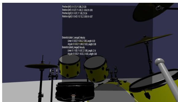
Figure 4: View of the velocity and position information displayed on the logger while drumsticks are held
