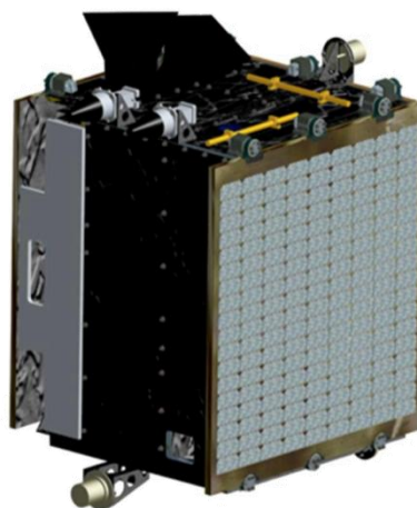
Figure 1: The PROBA platform with the PROBA-V instrument
