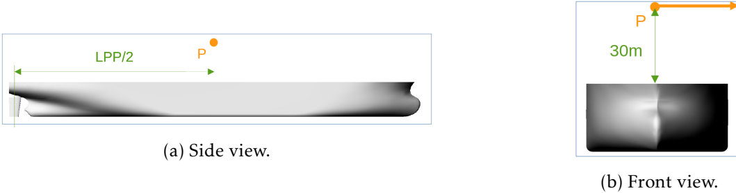
Figure 2: Point of application of the aerodynamic side force F_{y,WPS} in the case of the KVLCC2.
