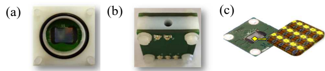
Fig. 1. Preliminary fabricated sensor: (a) top view of the sealed module, (b) assembled with emitter and receiver, (c) transducers mounted on a PCB with zoomed-in CMUT cells.
