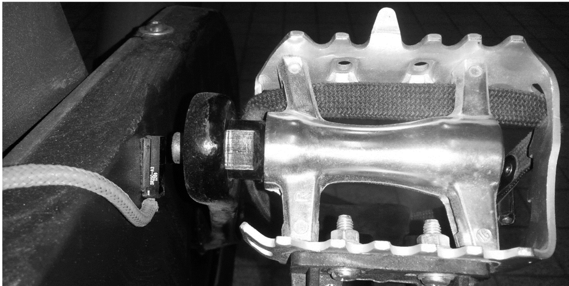
Figure 3. Custom synchronization setup with pedal-mounted magnet and frame-attached Hall sensor. Reproduced with permission from Billat et al., 2024 [43].
