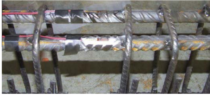
Fig. 3. Strain gauges attached to the steel bars.
