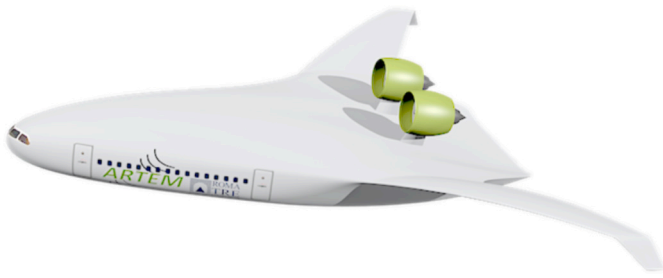
Fig. 2. Roma Tre University Blended Wing Body concept BOLT developed in H2020 ARTEM project (Grant Agreement 769359).
