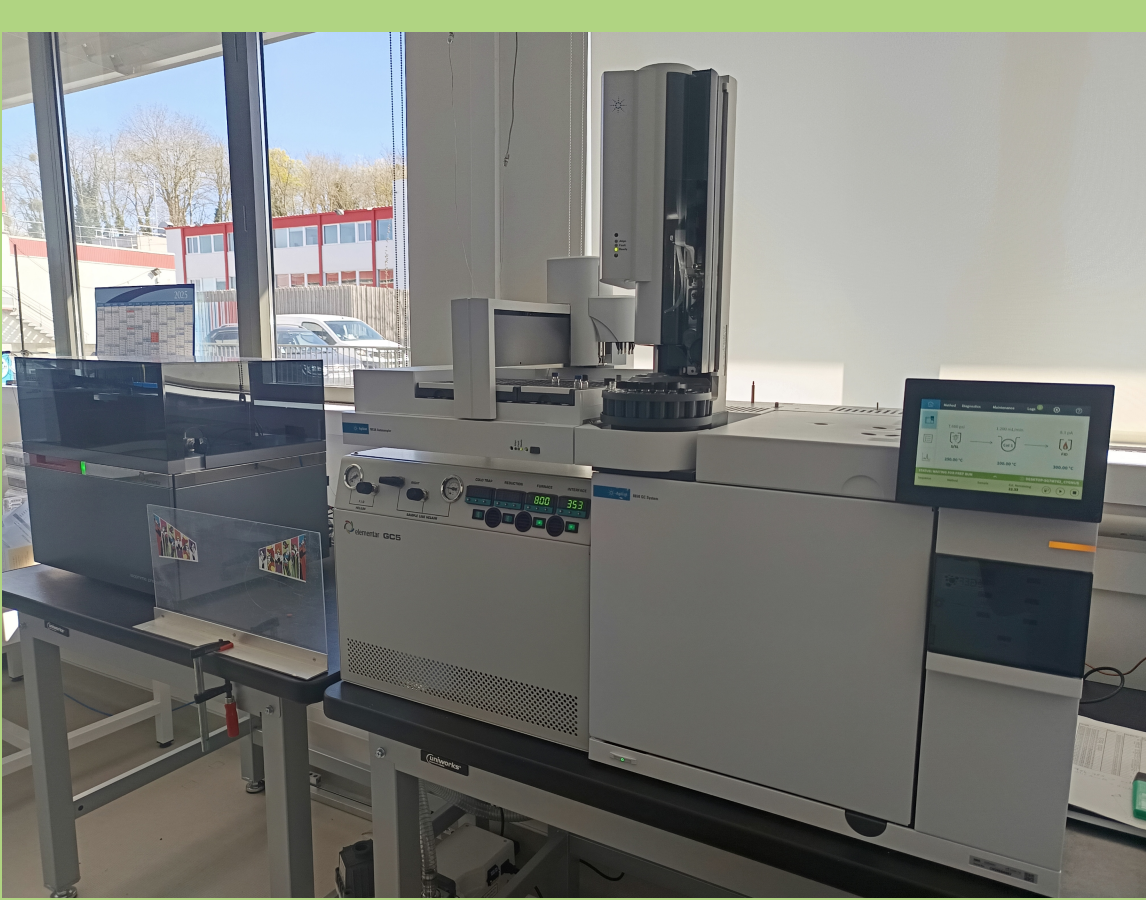
GC-Isotope Ratio MS for compound-specific 13 C and 2 H measurements
