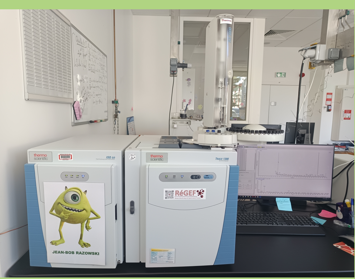
GC-Mass Spectrometry (MS) for lipid identification
