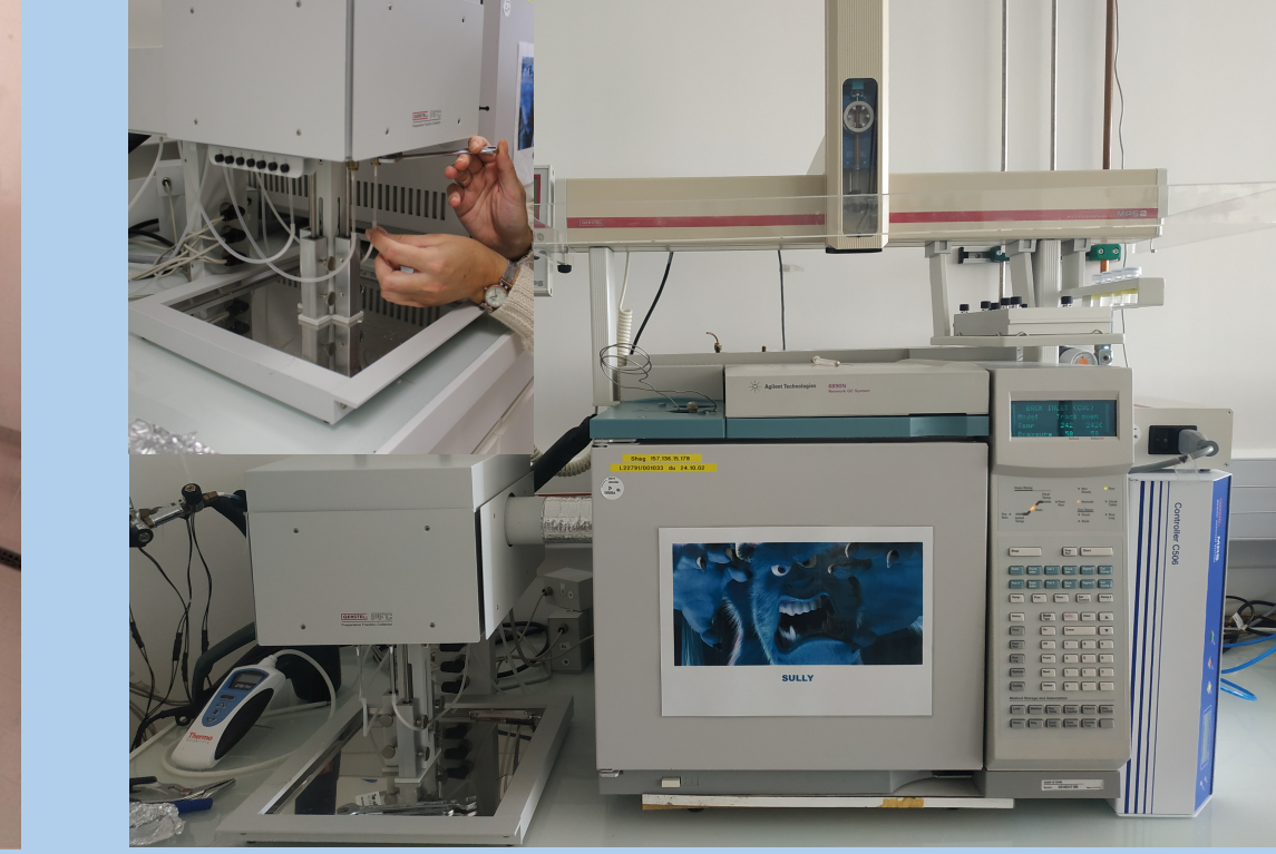
Preparative capillary gas chromatography for isolation of single lipids
