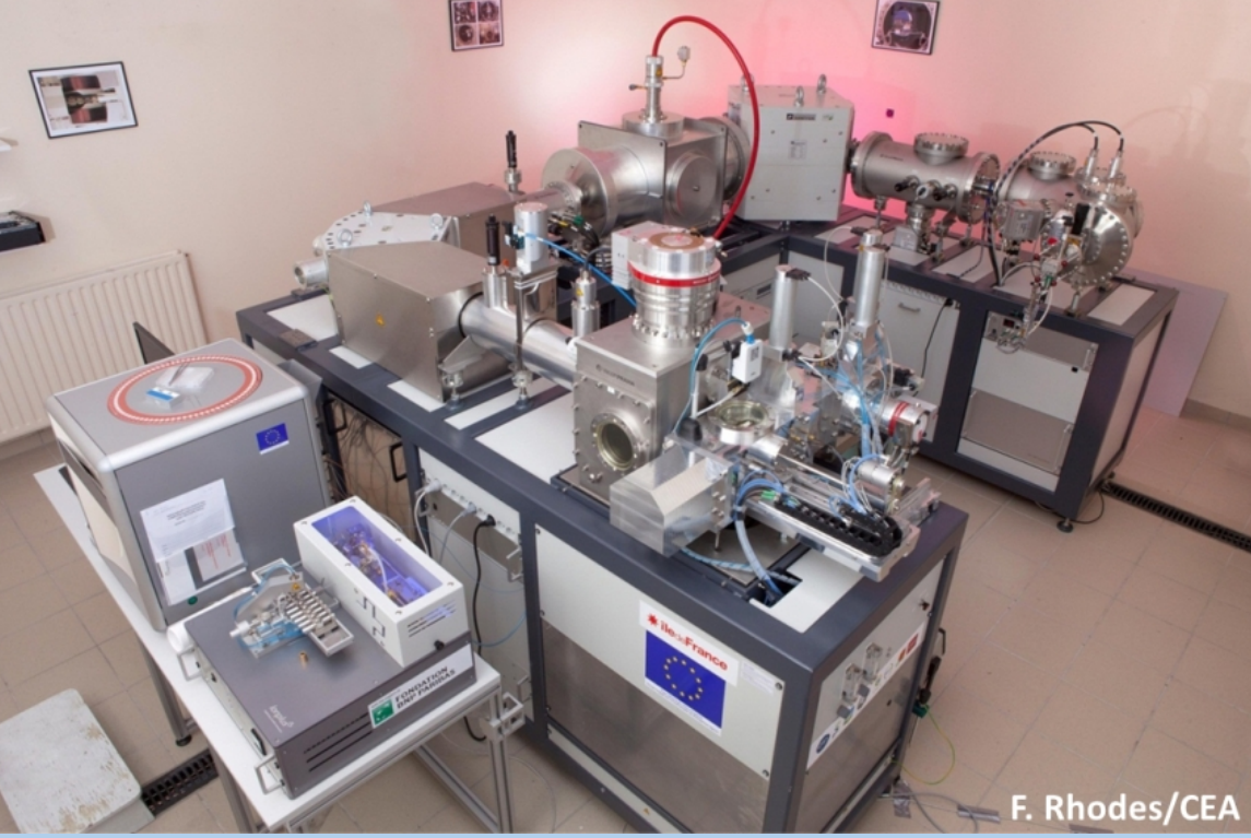
ECHO-Mini Carbon Dating System for 14 C measurement
