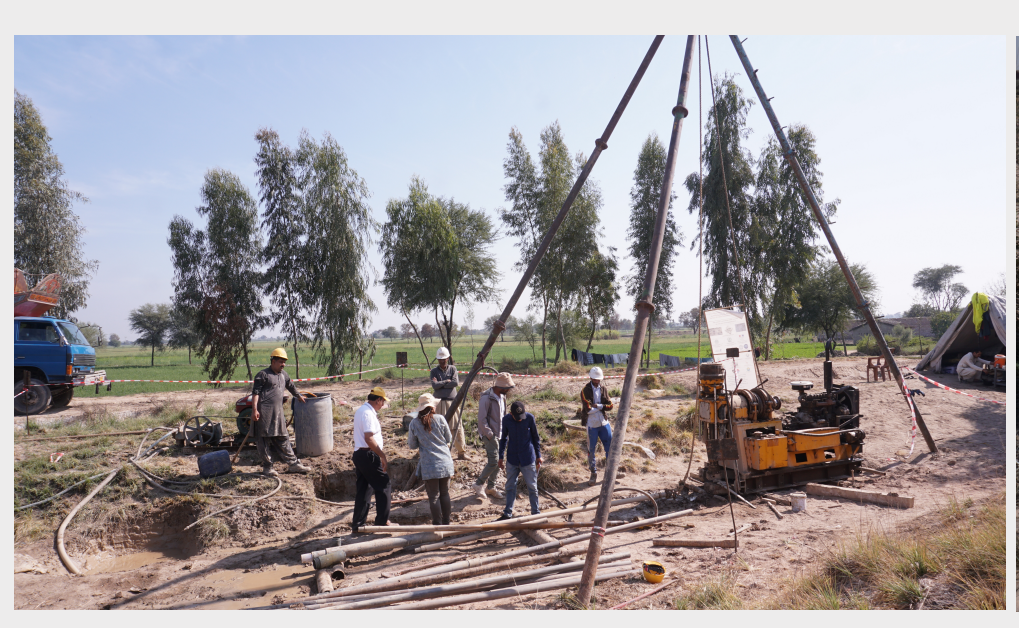
Coring of sediments
