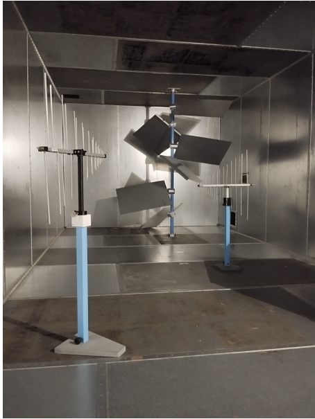
Fig. 1. IETR stirrer-mode reverberation chamber with the Tx and Rx antennas used for measurements.
