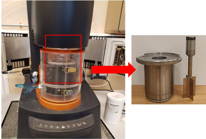
167 168 Fig. 4. The rheometer device and the vane-in-cup used geometry
