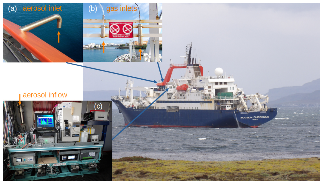
Figure 3. Picture of the Marion Dufresne in the Port-aux-Français bay (February 2024). (a) The aerosol and (b) gas inlets are located above the wheelhouse. (c) The acquisition and monitoring system is located in the meteorological room next to the wheelhouse and mounted above a shock-absorbing table. Aerosol monitoring systems are on the top shelf, to the right of the acquisition computer. Gas analyzers are on the bottom shelf. Photography credits: Meredith Dournaux.
