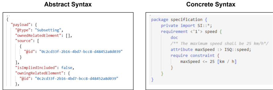
Fig. 2. Example of abstract syntax (left) and concrete syntax (right) in SysML v2 – The abstract syntax is the translation of the concrete syntax but was cropped for readability purposes.
