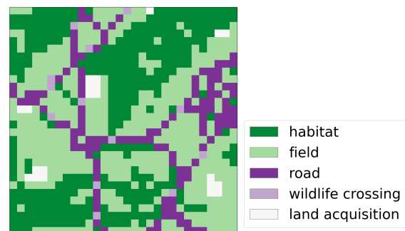
FIGURE 3 A 30x30 cell raster of a landscape on the outskirts of Aix-en-Provence (France) with roads on which wildlife crossings can be built and fields that can be acquired.
