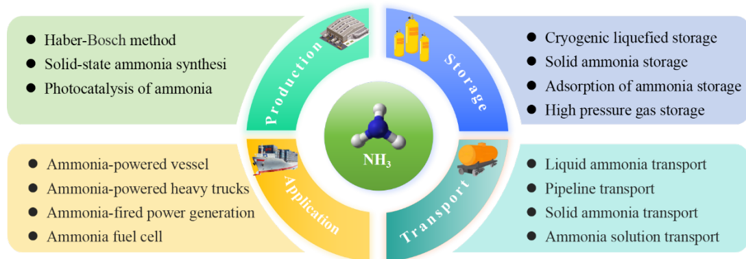
Fig. 1 The summary of the production, storage, transportation and application of ammonia
