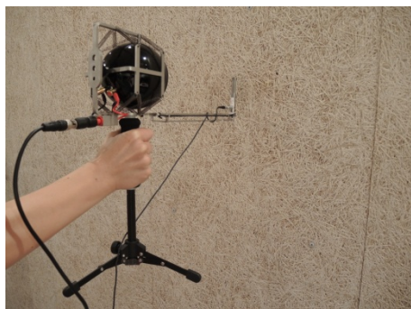
Figure 3 – Photograph of the p - v probe used in laboratory conditions for the determination of the absorption coefficient in-situ
