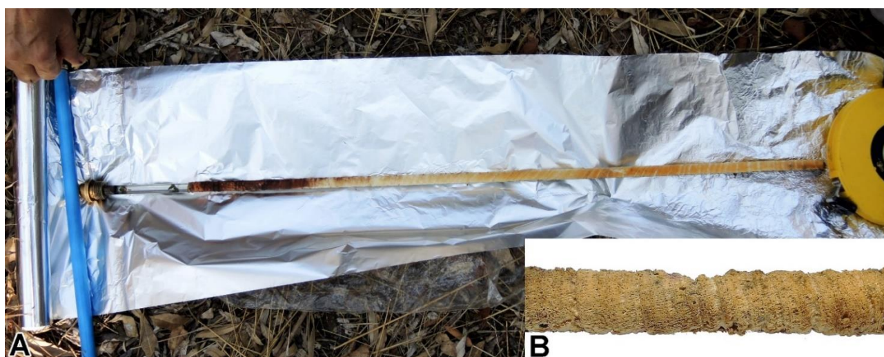
Figure 8. Photo showing sample A 257-1 being extracted from the increment borer to be wrapped in tin foil until further investigation (A). Detail of sample A 257-1, showing the growth rings, which typically become obvious 7–10 days after sampling (B).
