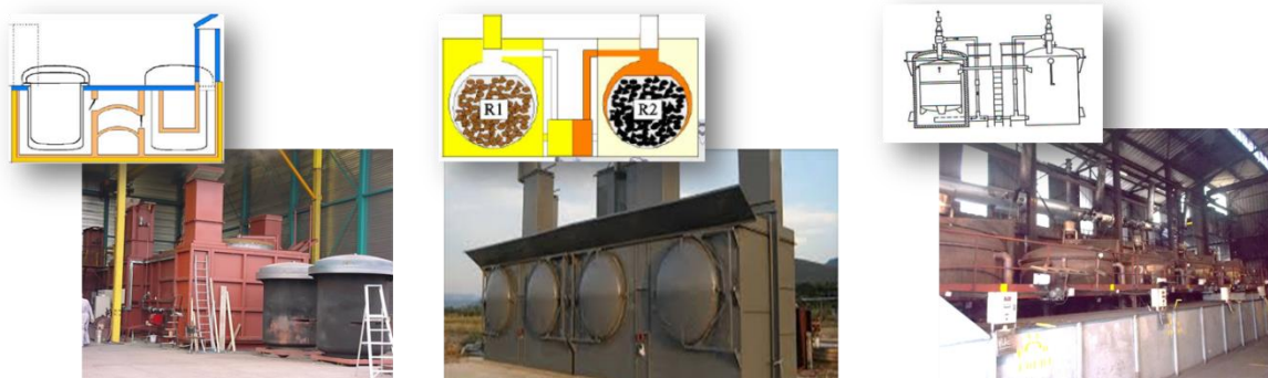
Figure 9. Charbon Engineering (Netherlands), VMR (France) and Sol Carbon (Belgium) technologies using external heating.
