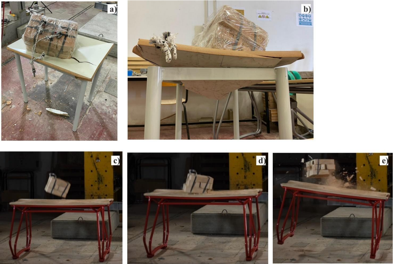
361 Figure 19. Impact test performed with a floor portion of 36 kg: a) traditional desk tabletop breach; b) traditional desk 362 tabletop-frame separation; c) impact on the life-saving desk; d) with energy dissipation; e) and overall bouncing.
