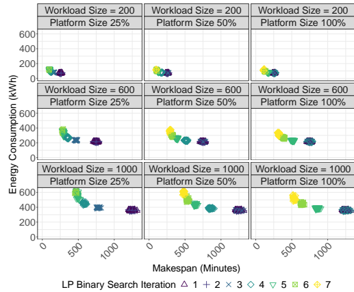
Figure 6: FOA-Energy Linear Program Pareto Front for the different combinations of workload and platform size.
