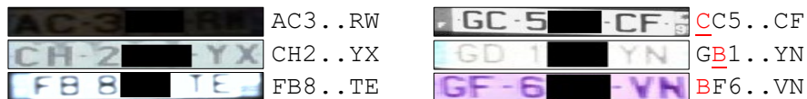
Fig. 1. Cropped photographs of real test LP with predictions by TrOCR. Left: Fine-tuned TrOCR successfully decodes images of LP starting with letters from A to F, (training-time syntax), despite degraded quality. Right: Yet, it fails on legible LP with a G in the leftmost position (future syntax). Errors (underlined) occur mainly in the first and second positions. LP are anonymised for RGPD compliance.
