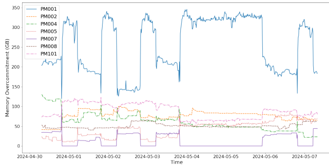
Fig. 15: Sum of ballooning, swapping and page sharing on each PM during deployment
