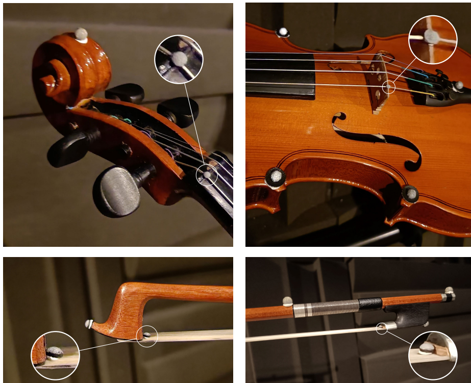
Figure 4: Markers placed at different points of the violin and the bow. The markers on the string and on the hair were used just for calibration, and removed for the test.
