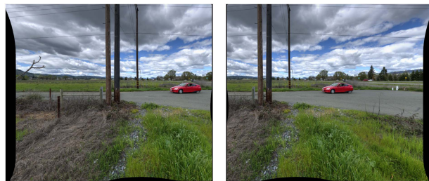
FIGURE 4. A sample of viewports extracted from a 360-degree image, with the image on the left illustrating the left eye's perspective and the image on the right illustrating the right eye's perspective. It is important to note that left and right view in Varjo VR-3 HMD do not completely overlap, making only part of the visual field binocular while the extreme periphery remains monocular.
