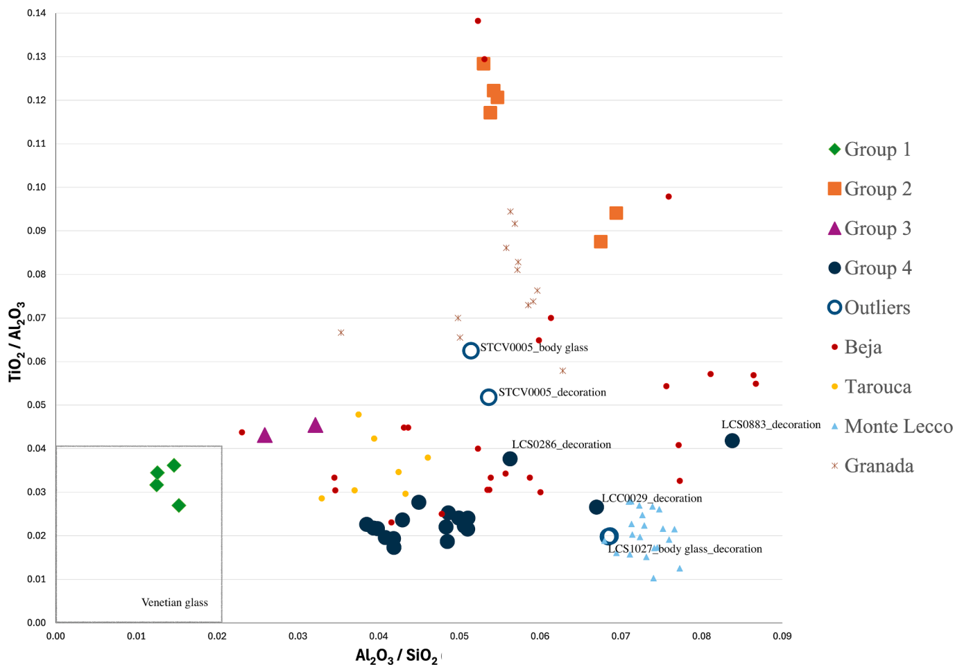
Fig. 7. Binary plot of weight ratio of Al_2O_3/SiO_2 vs. weight ratio of TiO_2/Al_2O_3 for the samples considered in this work together with the concentrations of glass unearthed in Spain, in Granada (Coutinho et al., 2021), and in Portugal in Beja (14th-16th cent.) (Coutinho et al., 2016a; Coutinho et al., 2016b) and in Monastery of São João de Tarouca (16th-17th cent.) (Coutinho, Medici, Alves, et al., 2016). The areas marked as Venetian glass refers to the cristallo and vitrum blanchum groups, considering values reported in Verità, 2013.
