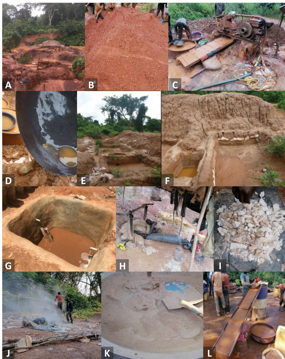
Fig. 2 Main ASGM practices in Kokumbo. A–B : exploitation of gold-rich river sediments and soils; C : device for washing alluvial ore; D : gold panning, E–G : cyanidation site. H : vein ore extraction shaft; I : crushed vein ore c; J–K : vein ore milling; L : vein ore flour washing ramp
