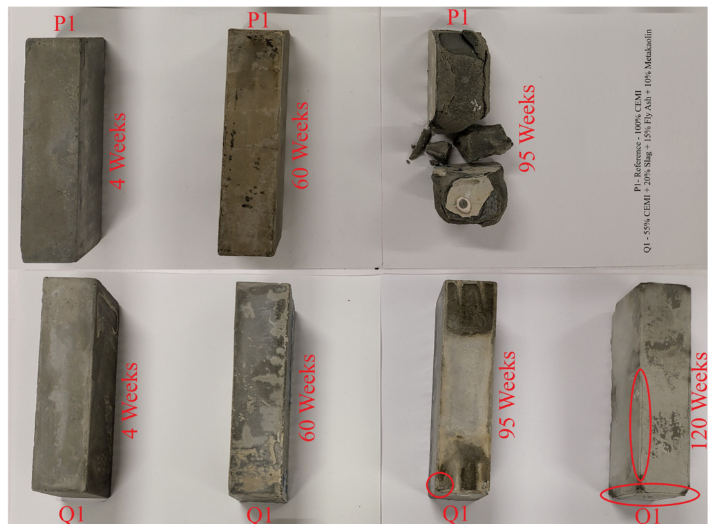
Figure 3. Visual inspection of P1 (reference mix) and Q1 after 4, 60, 95, and 120 weeks of exposure (the red circles highlight areas where cracks are observed in mix Q1).
