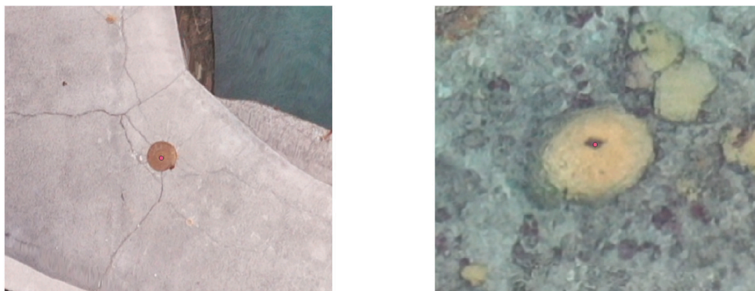
Fig. 5. Examples of Ground Control Points (GCPs) collected in Reunion Island in order to correct the aerial orthophoto position. Both human made objects (on the left) and easily distinguishable corals (a Porites coral on the right) can be used to set GCPs.
