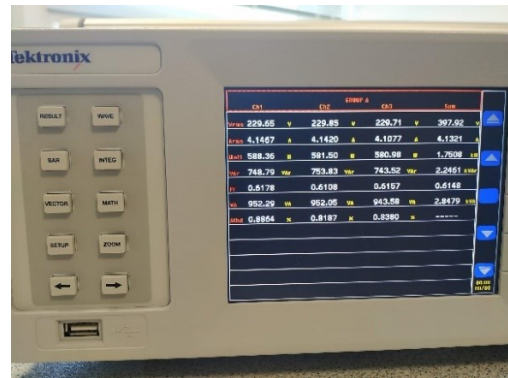
Fig. 18. Input power measurement for full load condition (PA4000).
