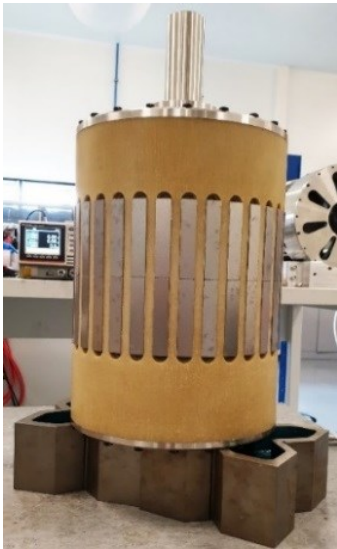
Fig. 6. Low speed rotor in G11 with ferromagnetic pole-pieces.
