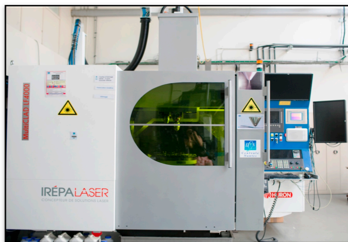
Figure 1. The IREPA Laser Direct Energy Deposition machine used in the study.
